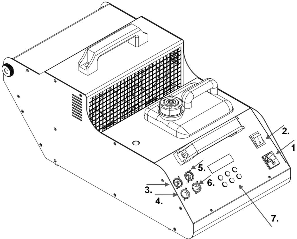
**1. POWER IN:** IEC current input socket with fuse holder for F6,3AL230V fuse.
