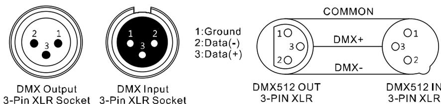
For installations with very long DMX cable paths or high electrical interference, such as in a discotheque, it is recommended to use a DMX terminator. The DMX terminator is connected in an XLR connector as a 120 Ω resistor between pins 2 and 3 which is plugged into the last output socket of the DMX line.
